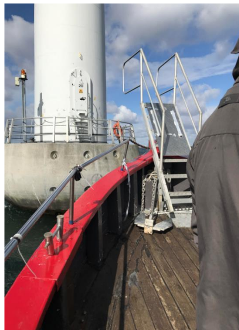
Figure 13: Maintenance is needed by the boat operator, like maintenance of the special access ladder from the boat to the top level of the foundation.
