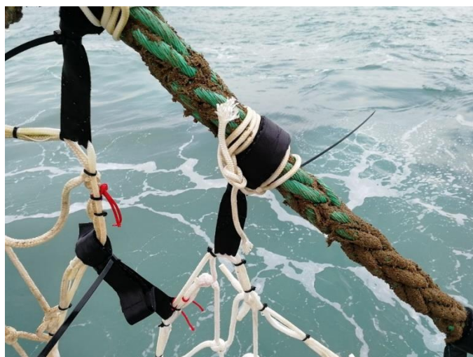
Figure 7: Velcro connection of nets to the backbone and the next following net
