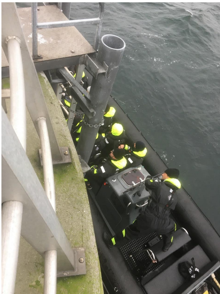
Figure 9: Approaching the foundation at sea level with a RIB Boat (Zodiac) can be a challenge when the wind speed is more than 8 m/sec and the current is not as the wind direction
